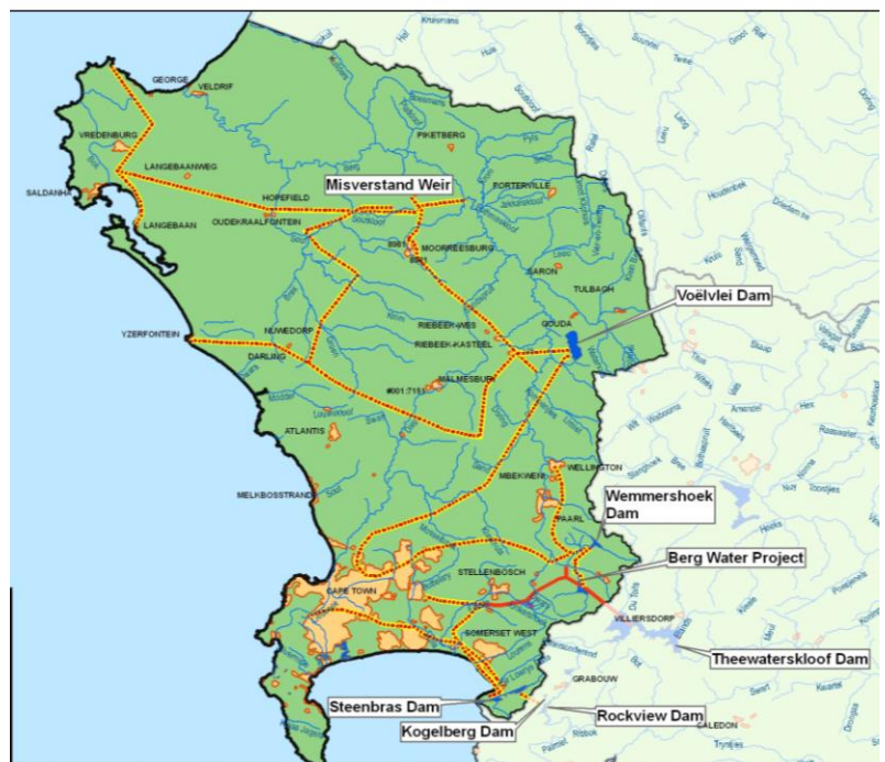
The map shows the main storage dams in the system, and how all these are connected to one another in order to operate the system at its maximum efficiency so as not to let any dam spill unnecessarily
